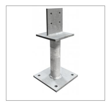
The PBH is suitable for heavy duty post support applications including Glulam timber posts with a standoff height of 200mm. Dowels included. PBH75 suitable for posts 75 x 75mm to 120 x 120mm. PBH120 suitable for posts 120 x 120mm to 200 x 200mm.
