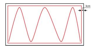
Wait for a couple of minutes and then press boards strongly onto substrate (within 8 minutes from extrusion, 20°C, 65% r.h.). At higher temperatures/humidity, the open time
