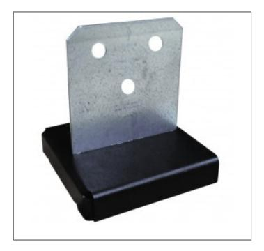
The CPT concealed post base provides a clean, concealed look while providing a 25mm standoff height above concrete. The 25mm standoff reduces the potential for decay at the post end. The CPT can be fixed to concrete base with either M12 chemical or mechanical anchors (sold separately).
