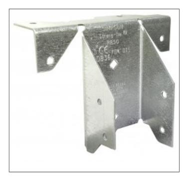
The RR ridge rafter connector provides alignment control and correct nailing locations. The RR may be used with any rafter slope up to 30°. For back-to-back installations, the minimum width of the ridge plate is 38mm.
