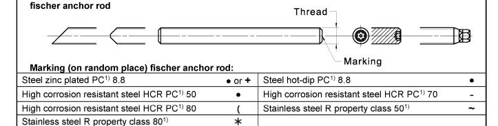
Alternatively: Colour coding according to DIN 976-1: 2016
